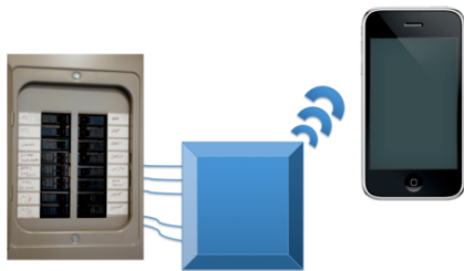
Figure 5 Circuit breaker box, data collection hub, iPhone
